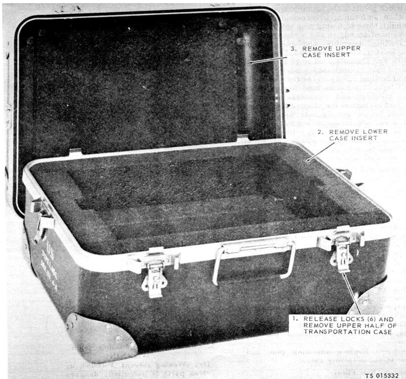
Figure 4-6. Transport case inserts, removal and installation.
